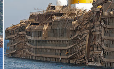
Crushed starboard side of the righted ship
